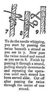
The hemp thread which saddlers and shoemakers use is the best stuff to use for whipping, about three thicknesses worked up together with cobbler's wax or beeswax will stand anything, being much stronger than ordinary twine.
