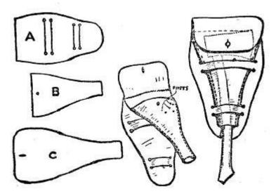
A – shows the shape of the back piece of leather. Eight holes are punched in it, which are joined by slits cut in the leather. B and C form the case proper. B is placed on C and stitched, leaving the top part of C quite free. Slip the axe into the case, then put in rivets to prevent the stitches being cut. A is sewn on to the back, and the case is slipped through the "straps" of leather in A. Finish by making a fastener to keep the case closed.
