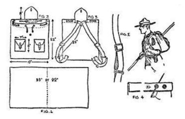
Figure 1 shows the length of material required. It is folded, and sewn up at the bottom and along the side, making a kind of bag. Sew on the flap, make the holes for the cord, and stitch on the straps. Figure 4 shows you how to sew round the eyelet holes.
