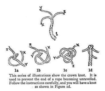
You begin by unlaying the rope a sufficient distance, which is roughly about ten tunes its thickness (a rope  $\frac{1}{2}$  in. thick would be unlaid about 5 or 6 in.). Be very careful about this unlaying, and keep a hold on the strands so that they will not lose the twist which gives them their strength.
