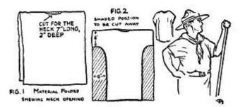
You first of all obtain your piece of material and double it (fig. 1). Cut the neck-piece and form the sleeves by cutting the pieces shown by the shaded parts (fig. 2). Hem and stitch together, and your shirt is complete.
