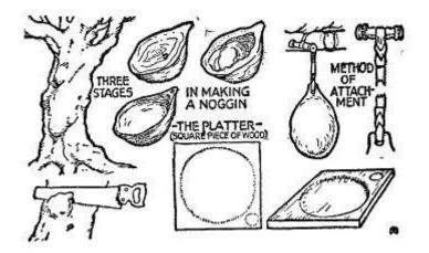
When you have found the ideal "bump," on a suitable tree, saw it off. Having done this, scoop out as much wood as you can, leaving the cup about ½ of an inch thick. To hang the cup to your belt, bore a hole in the wood, and attach by means of a piece of rawhide. To make the wooden "platter," get a piece of wood about a foot square. Scoop the wood from the centre. The small hole in the corner is for such things as salt.
