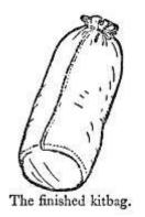
That finishes the body. Turn it inside out and now you have a canvas tube open at each end. Take another piece of canvas, similar to that in figure 3, and draw two circles on it, using pin, pencil and piece of string to make the lines, one 12 in. in diameter and the other 10 in. Now cut round the outer circle.
