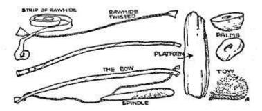
The sketches clearly explain how to make your fire set. The twisted raw-hide is fastened to a stiff piece of wood two feet long to form a bow. The platform is a piece of elm, as also is the spindle. The palm is a stone with a hole in the centre, or you can make one from a knob of wood. The tow is made by fraying a piece of rope.
