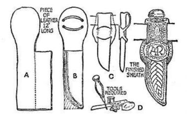
(A) shows the rough shape to which you must cut the leather. You next fold at the dotted lines, then sew as shown in sketch (B); also cut the slits depicted at the top. (C) shows the method of fastening the sheath to the belt. (D) shows the tools you require, and finally you have the finished article.
