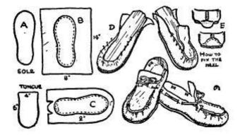
Cut out the sole, and place it on the underneath of the leather as illustrated in B. C shows you how to shape the "upper." Place the dummy foot inside the "upper," draw the leather over, and tack round as in D. Now cut out a tongue and sew inside as illustrated in the right-hand picture of D. E shows you how to fix the heel. Then finally you see the finished moccasins
