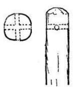
Figure 3.—To find a right-angle with your staff bore two holes straight through it at right - angles. This article tells you how to use it.
