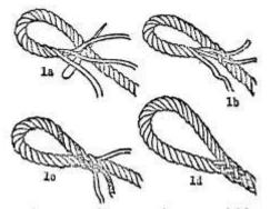
Diagram 1a shows you the rope unlaid ready for splicing. In 1b you see the left-hand and middle strands worked into the main rope. In 1c the right-hand strand is shaded, having been brought across the back of the splice. 1d shows the finished splice.
